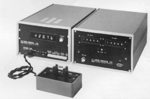
also appear on a rear panel connector as open-collector TTL logic states (+5V, true; 0V, false) and as relay closures for each limit.
