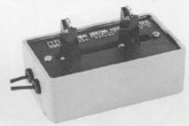
This fixture holds components for test while providing four-terminal connection. Its holding clips can rotate 90 degrees to accommodate axial and radial-leaded components. They can also be set from 116cm (5/s in.) to 8cm (3½ in.) apart. This allows use of this fixture with many component sizes and configurations.
