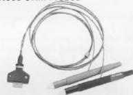
The small, spring-loaded tips of the OHM probes are designed for getting into small, hard-to-reach spots. They are especially useful for probing circuit card components, reaching connector
